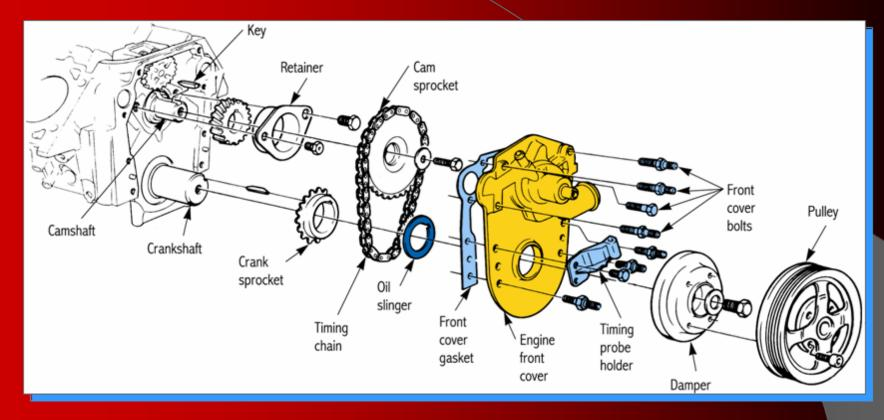
Holds the front oil seal, timing pointer, probe holder, and other parts Engine Front Cover
