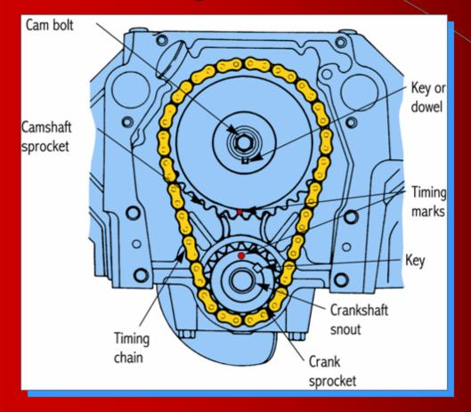
Timing marks must line up to time the camshaft with the crankshaft
