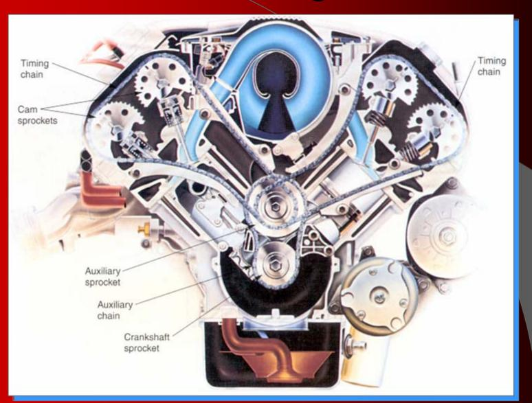
Auxiliary Chain • May be used to drive the engine oil pump, balancer shafts, and other units on the engine
