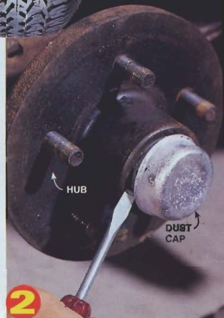
Remove the grease cap carefully. You'll reuse it.
