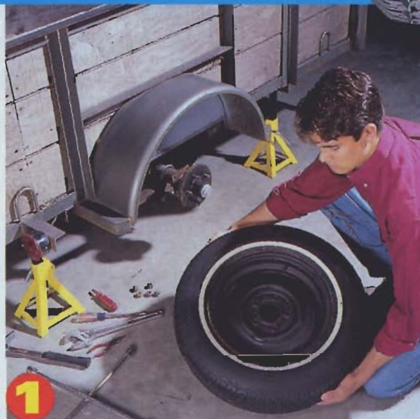
Remove the lug nuts and the wheel. Be sure the trailer is supported with jack stands.
