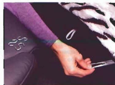
3 Push the elastic straps through the gap between the back and the seat bottom.
