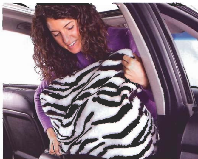
2 Determine which cover is the driver's and which is the passenger's side (most universal covers are the same). Slip the cover over the back and wiggle it down like a tight sweater until the top fits snugly.
