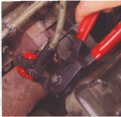
3 Using a wire puller, twist the boot to break the seal from the plug and then pull off the old plug. Match the old wire length to the new wire.
