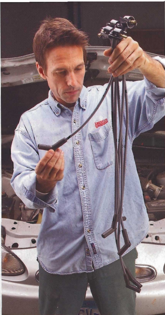
2 Uncoil the new spark plug wires and sort them by length.
