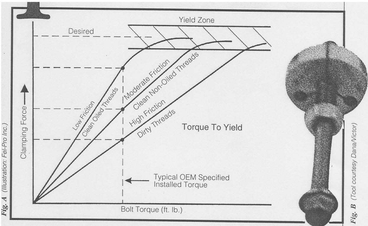
**Fig A.** Although the torque-to-yield procedure provide a more uniform clamping force, it permanently stretches the bolt. Reusing stretched bolts can lead to sealing (gasket) problems, which is why using recommended TTY bolts is highly-recommended.
