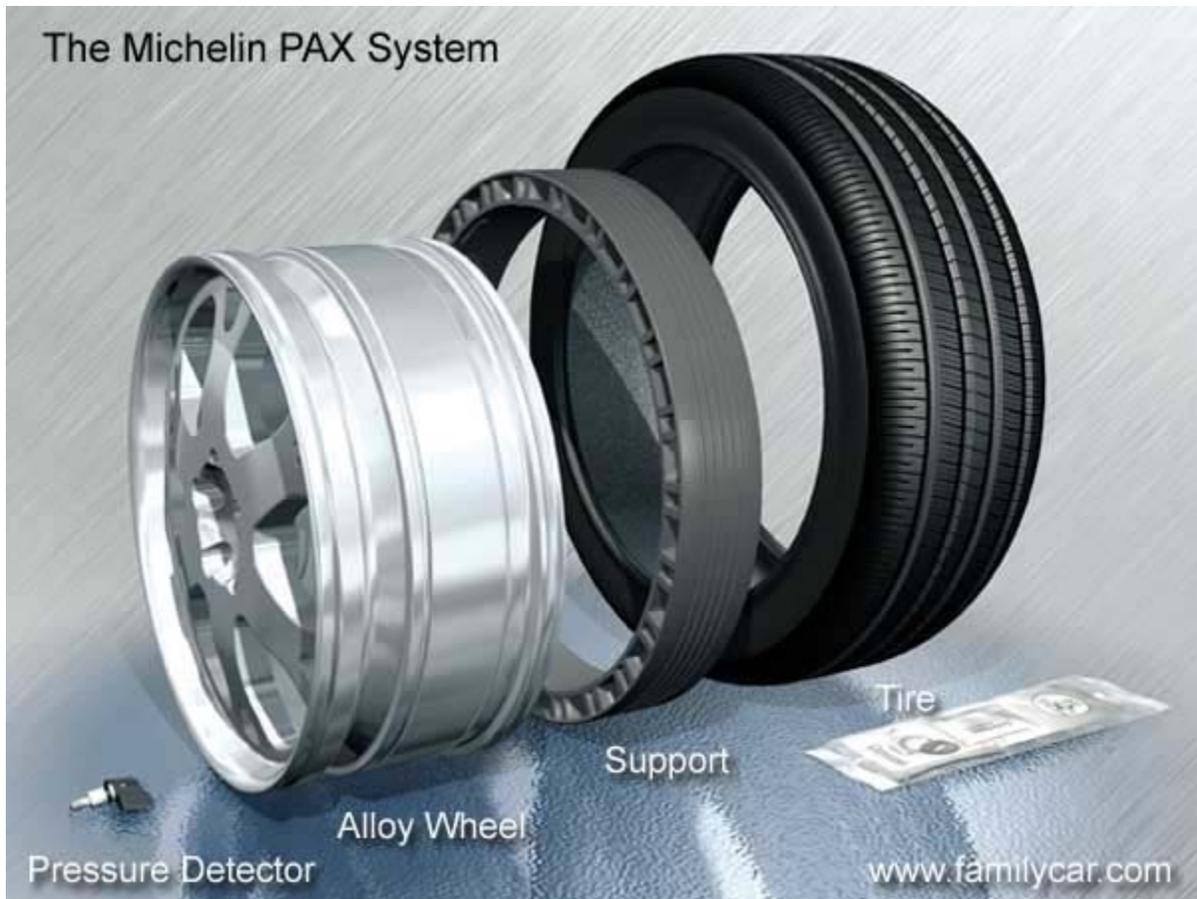
The PAX System includes a special wheel and tire that are designed to work together. There is also a support ring that fits around the center of the rim and supports the tire when it is deflated so that the vehicle can be driven. Another part of the system is the combination air valve / pressure detector which reports pressure loss to an indicator on the dash so that the driver knows that there is a problem.
