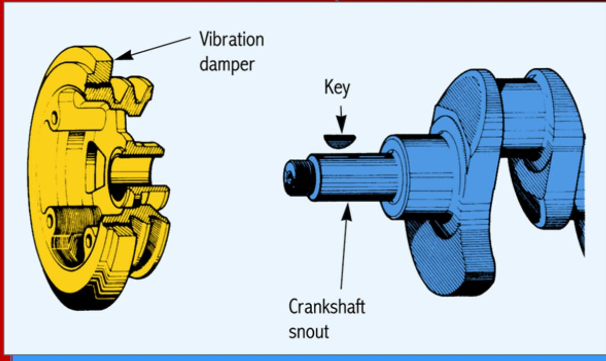
Constructed of a heavy wheel
