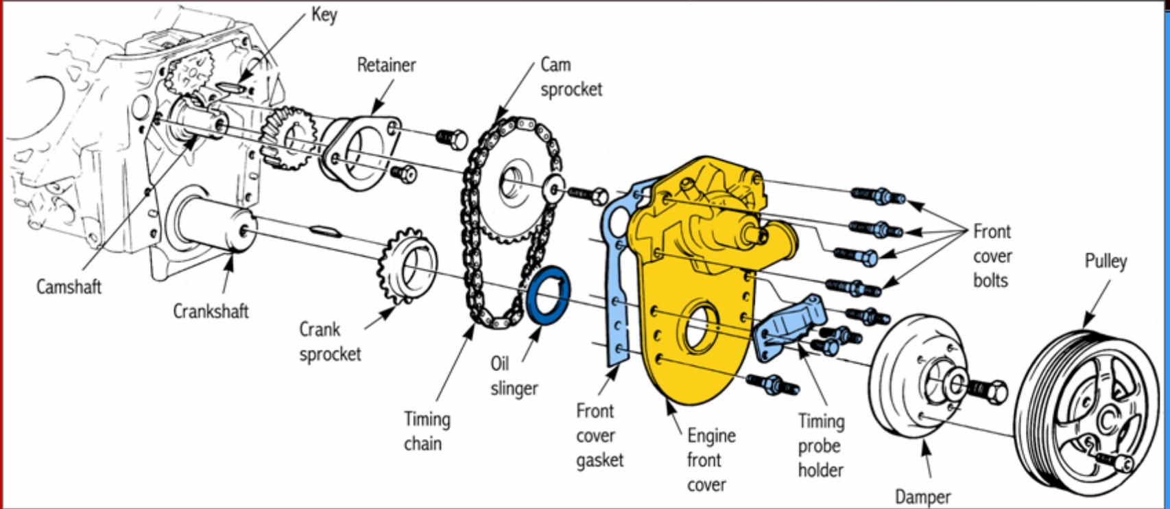
Holds the front oil seal, timing pointer, probe holder, and other parts
