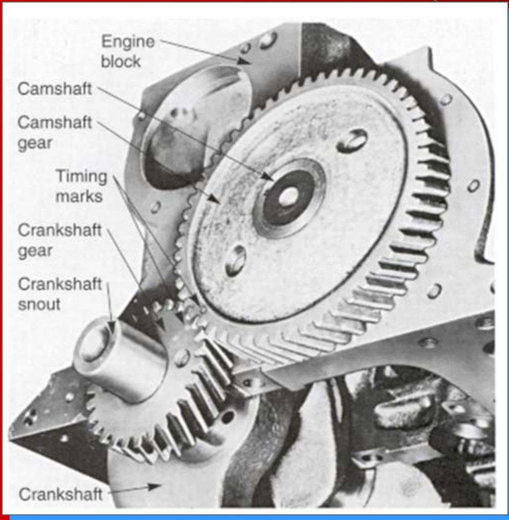
Timing marks show the technician how to install the gears properly
