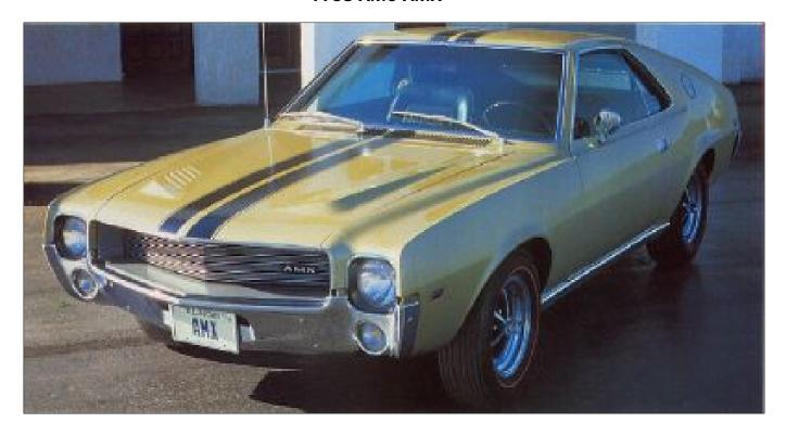
The AMC AMX debuted on Feb. 24, 1968, as a midyear 1968 model. It was the first steel-bodied, two seat American production model since the 1957 Ford Thunderbird. American Motors created the AMX (American Motors Experimental) by slicing a foot out of its Javelin body, eliminating the rear seat, and making it a true two seat sports car. Its short 97 inch wheelbase cut the AMX curb weight to about 3,100 pounds.
